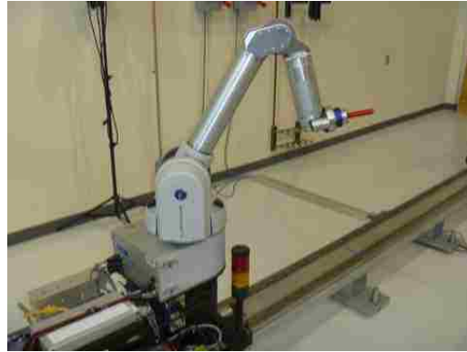
Figure 5.1: Whole Arm Manipulator (WAM).
